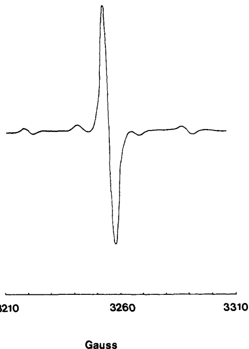
Figure 2. ESR spectra obtained from in situ electrolysis of Cr(CO) 6 in dichloromethane (saturated Bu 4 NClO 4 ) at -80 °C.
